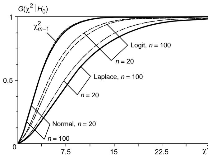
Fig. 2. Distributions for the Bartlett statistic when the observed parameter differs from a normal distribution for various sample volumes and  $m = 5$ .
