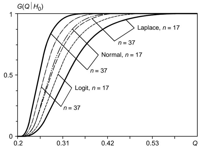
Fig. 5. Distributions for the Cochran statistic for deviations in the distribution of the observed parameter from normal with various sample volumes and  $m = 5$ .
